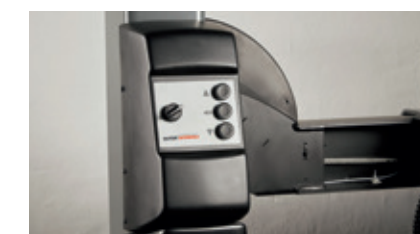
Pump and control unit on front left post
