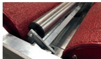
Sensory rollers of stainless steel
