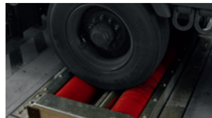
Sensory rollers of stainless steel
