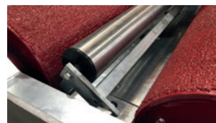
Sensory rollers of stainless steel
